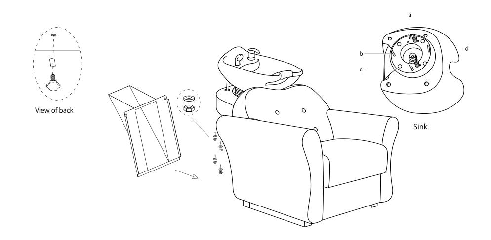
Undo the access panel by twisting clockwise then using the 4\* 14mm washers & gaskets provided fasten the sink to the base.
