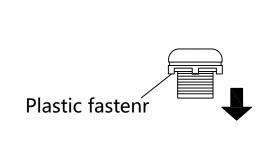
Unscrew the fastener from the sprayerhead holder.
