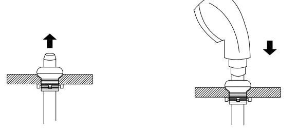
Place the sprayer hose from underneath throught the sprayerhead holder and fasten the sprayerhead to the sprayer hose.
