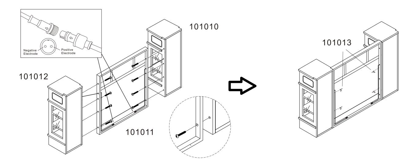
The connectors of the black wires are connected to each other, and the connectors of the white wires are connected to each other
